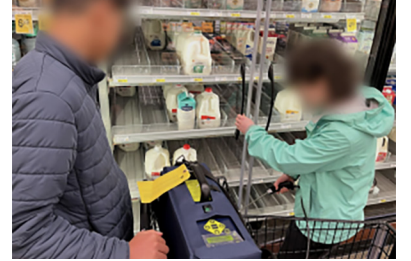
Detecting leaks with the Gasmeter in a grocery store aisle
